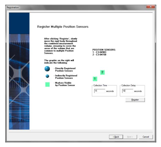
Collection time is default 15 seconds. Collection delay will give you some time to go from the computer into the alignment area. The '1' and the '2' should both have green squares, meaning that both position sensors see the cube. After pressing the 'Register' button, make sure to move the cube in at least a 1 meter by 1 meter by 1 meter space. And make sure that there are enough samples where both position sensors see the alignment tool.
