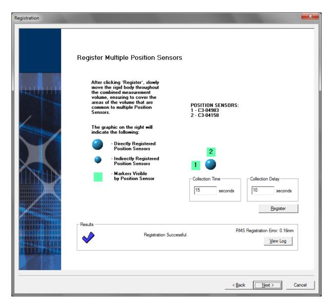
Registration is successful. RMS Registration Error tells the accuracy of the registration. Lower is better. The RMS registration error should always be below 0.3 mm.
