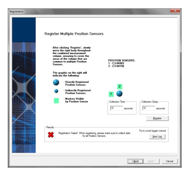
Registration failed. Try again and make sure that the alignment tool is moving in at least a 1 meter by 1 meter by 1 meter space and that both position sensors see the cube.
