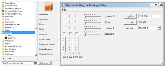
First the 'Beer' program automatically looks for the Behringer mixer to make a connection (see.get ip: 192.168.1.1). After the connection has been set up the program initializes (resets!) the Behringer (see.use:192.168.1.1) automatically.
