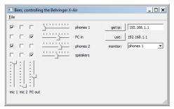
In this example the 'mic 1' is used at maximum volume sensitivity. The output of this device goes to 'phones 1'. Because the volume control of 'phones 1' is at its lowest level no sound will be available on the headphones 1. Also the input device ('mic 1') goes to 'phones 2', here the sound level has been raised to 62 and audio will be played.
