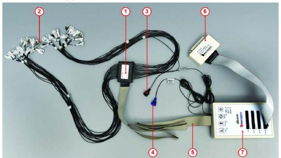
Remove the splitter box hanger from the stand and place it next to the sink in the white insert. Make sure that the splitter box and connection cable (no 1 and 5 in figure) are kept dry at all times!
