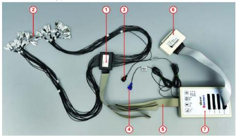
Remove the splitter box hanger from the stand and place it nest to the sink in the white insert. Make sure that the splitter box and connection cable (no 1 and 5 in figure) are kept dry at all times!
