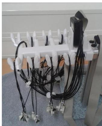
**Clean the electrodes (electrode tips and side opening of the electrode head)** with a *toothbrush* using *lukewarm, running water*. If the electrodes have a tubular space, make sure to clean it with a *needle or tooth pick*! While doing this hold the electrode by the head, not the very tail of the plastic part and **not the wire!**
